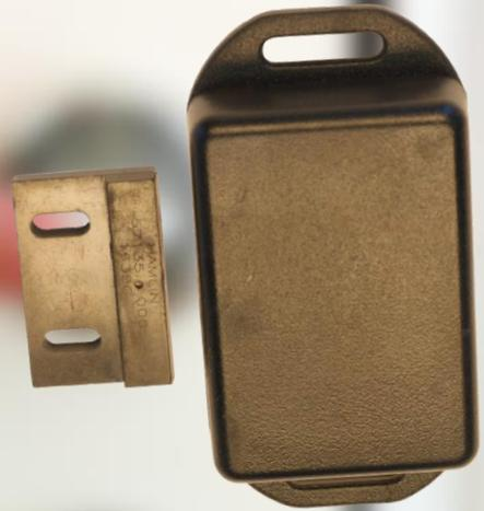
TWIG Door Sensor is a short range device (SRD) designed to improve safety of TWIG personal alarm users e.g. security guards and maintenance workers by registering their comings and goings at door openings.
