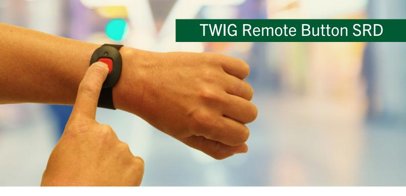
TWIG Remote Button is a short range device of SRD transceiver category 2, designed to be worn on the neck, on the wrist or in the pocket. Paired with a nearby SRD or SRD3 -enabled TWIG personal alarm device as its base station, it enables remotely launching MPTP protocol messages with a single push of button.
